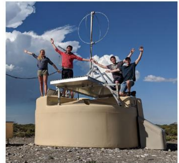
Water-Cherenkov detector (WCD) with new surface scintillator detector (SSD) and new radio antenna.
