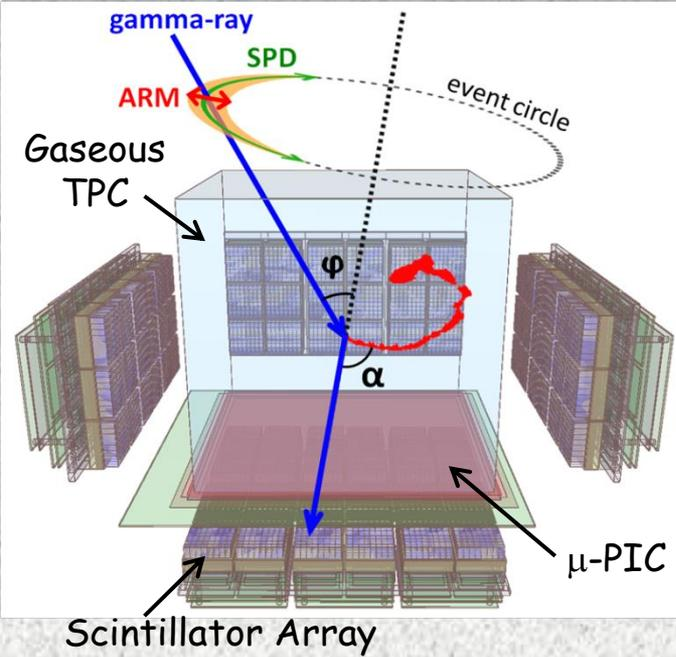
30cm-cubic Gaseous Time Projection Chamber
